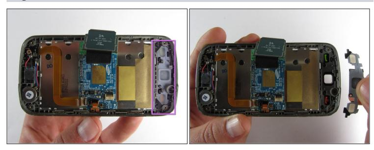
• In this procedure, the rubber function key pad can easily fall out, so it would be best to take it out and set it safely aside.
