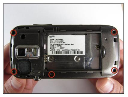
Remove the five 3.4mm Philips screws securing the backing of the phone.
