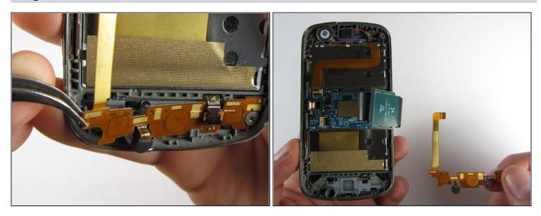
• Using tweezers, gently remove the bottom orange strip from the device
