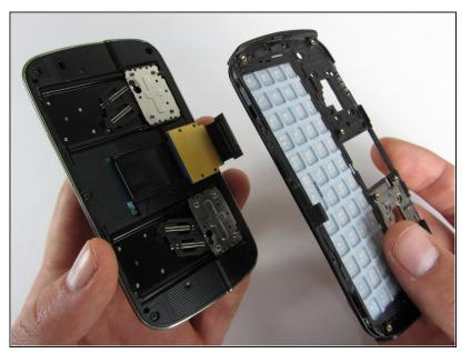
Carefully remove the keyboard frame from the sliding mechanisms underneath.
