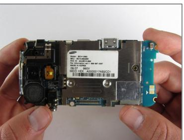
• Use a plastic opening tool to disconnect the film from the motherboard.
