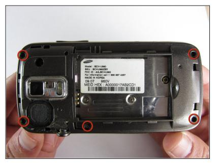
Remove the five 3.4mm Philips screws securing the backing of the phone.
