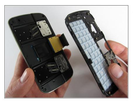
Carefully remove keyboard holder from the slider mechanisms underneath.
