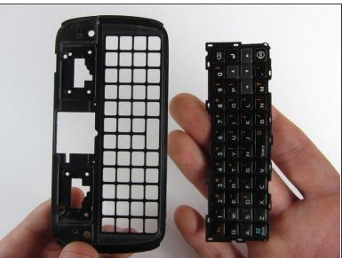
Turn keyboard holder over and allow the keyboard to simply fall out into your hand.
