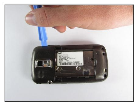
Use a plastic opening tool to carefully pry the back cover surrounding the camera up from the phone.
