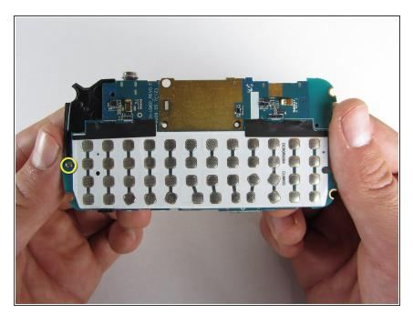
On the underside of the motherboard, remove the single 3.3mm Philips screw.
