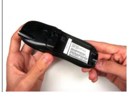
Remove the battery by pushing the bottom end towards the top, then lifting up.
