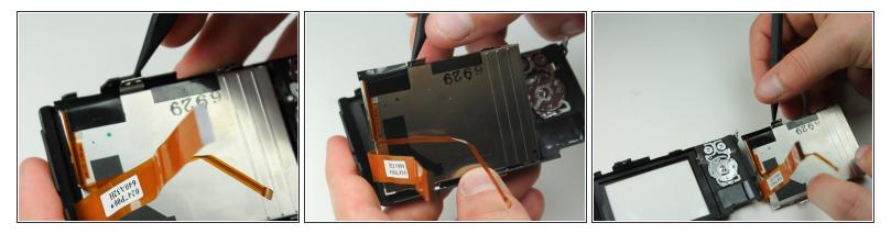
Use the pointed end of the spudger to pry off the LCD screen from the back cover. Place the tip of the spudger in the small hole in the bracket on the LCD screen and lift it out.
