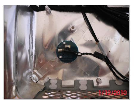
• To get to the power button first remove the hard drive fan as seen in other guides.
