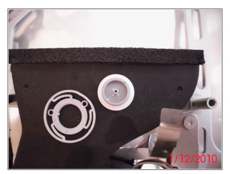
• The center of the washer has a center locking pin to correctly place it on the back of the button. The washer is concave and the concave side faces the button, This gives the button a spring to it so that it will pop back out.
