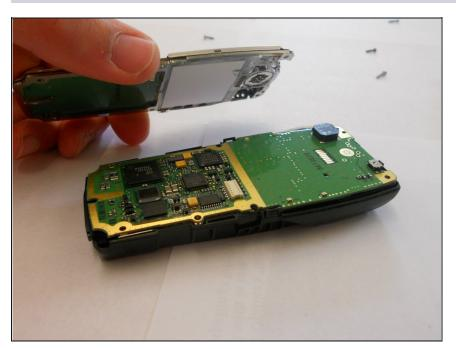
Set the screen carefully over the body of the phone, avoiding any sliding on the Logic board
