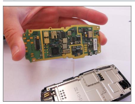
Insert in the replacement Logic Board, setting the Logic Board carefully back into place.
