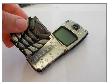
• Replace keypad onto the device
