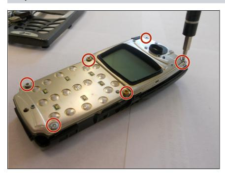
Replace screws in the corresponding slots, tightening them till they are not loose.
