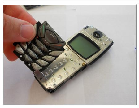
Simply remove the keypad from on top of the phone, and place it off to the side, leaving just the phone itself remaining
