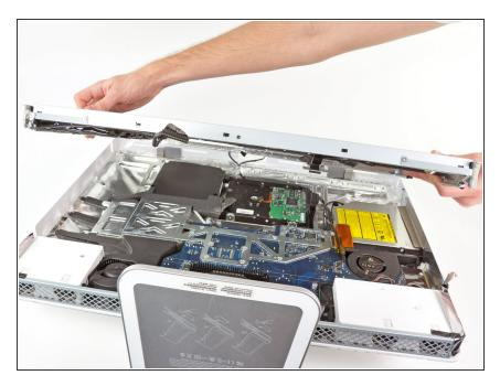
Remove the display assembly from the iMac.
