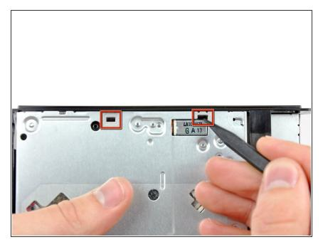
Use the tip of a spudger to push the two optical drive bracket tabs out of their slots in the top of the optical drive.
