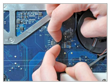
Pull the optical drive thermal sensor connector toward the right side of the iMac to disconnect it from the logic board.
