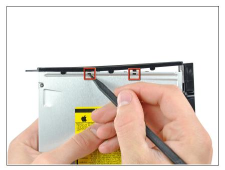
Use the tip of a spudger to press the optical drive bracket tabs out of the slots in the top of the optical drive.
