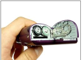
When finished, you should have one battery positive side up and the other one negative side up.
