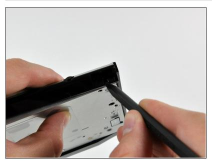
Using the sharp end of a spudger, press the optical drive bracket tab out of its slot on the side of the optical drive.
