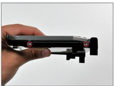
• Remove the two T10 Torx screws from each side of the optical drive (four screws total).
