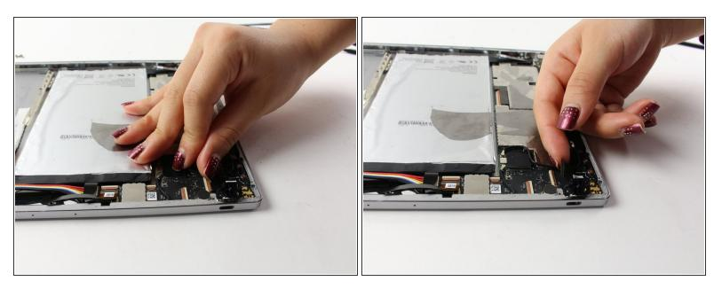
Detach the larger connector wire by flipping the copper hinge located at the base of the connection with your fingernail.
