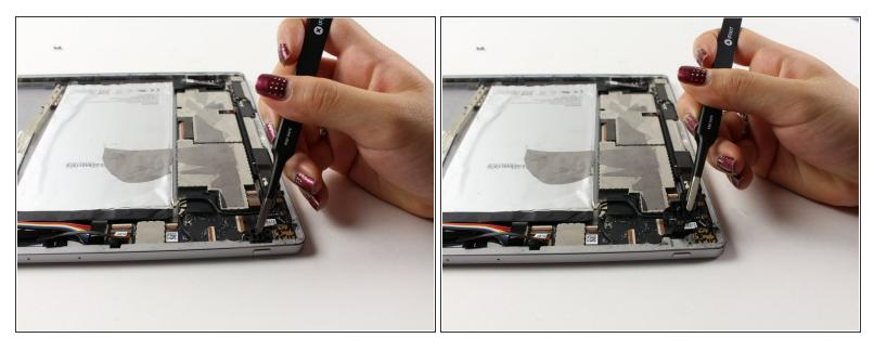
Use tweezers to slowly pull up on the power button technology as far as possible without pulling out the two black wires attached.
