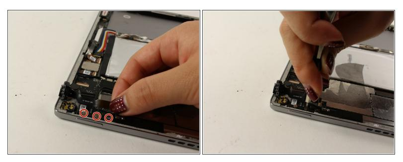
Locate and remove the three 4.2mm Phillips #000 screws at the base of where the second wire is still connected.
