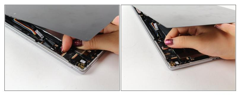
• Detach the cables for the camera by lifting the small flap using the tip of your fingernail or a spudger. Gently pull the ribbon cable out.
