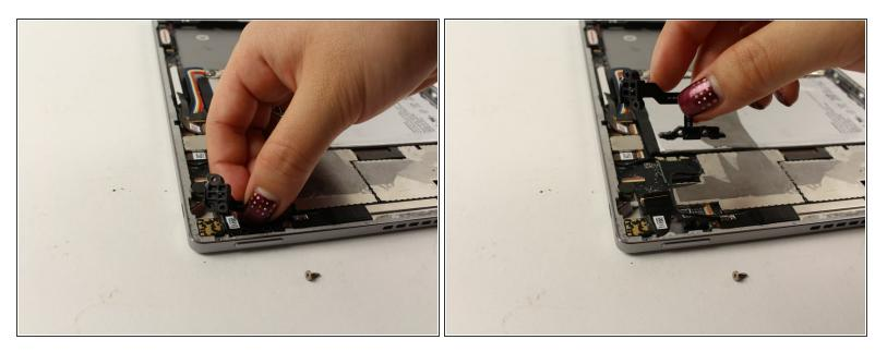
• Once all the screws are removed, gently pull up on the entire power button technology piece, to remove it from the device.
