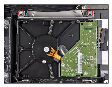
Remove the two T10 Torx screws securing the upper hard drive bracket to the outer case.
