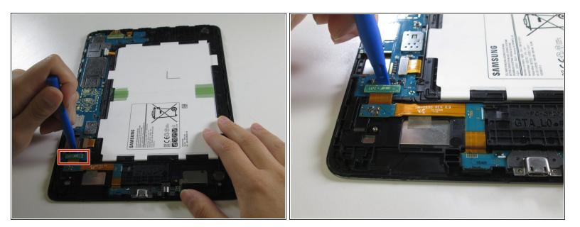
• Use a plastic opening tool to pry the two connectors near the charging port from the motherboard.
