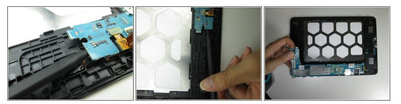
• Using your fingers or a spudger, gently remove the motherboard from the device.
