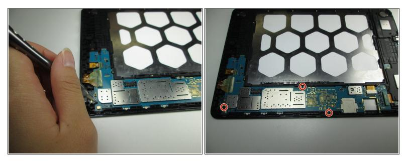
Use a #000 Philips screwdriver to remove the three 2.8mm screws attaching the motherboard to the device.
