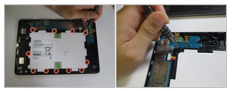
Remove the eleven #000 Phillips 2.8mm screws that hold the battery in place.
