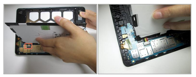
• Pull the battery out until it is only connected to the device by the black, yellow, and red connectors.
