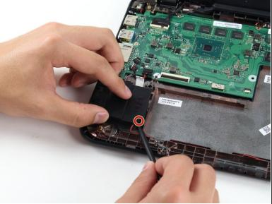
Use the pointed end of the spudger to pop the speaker up and off of the two posts.
