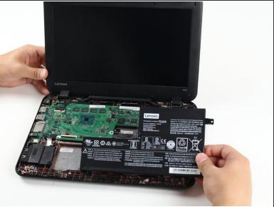
Lift up on the tabs that were held down by the screws to remove the battery.
