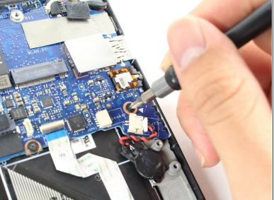
Remove the eight 4 mm Phillips #0 screws from the motherboard.
