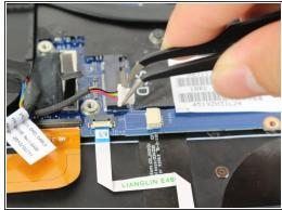
• Use tweezers to remove the little white connector by pulling it out and away from its socket.
