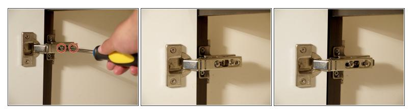
(i) Use this step to adjust the amount of space between the cabinet door and the cabinet frame.
