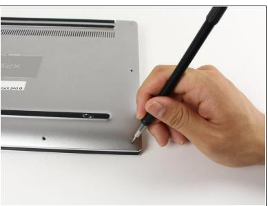
Remove the eight 4 mm T5 Torx screws from the bottom cover.
