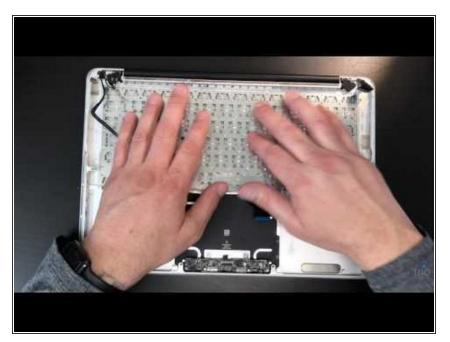
Inspect Keyboard and Track Pad for ANY corrosion or sticky residue – If found a keyboard or trackpad replacement is recommend.
