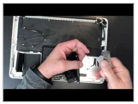
Batteries are often victims of liquid spills and can be very challenging to replace. Battery installation varies from model to model. Here is an example of what you can expect.
