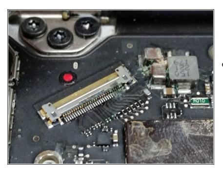
All display connections and wiring should be throughly inspected, any sign of liquid exposure and the display replacement recommended. If you see something like this, you may have issues with the display. Remember, all MacBook displays are sealed units and require advanced equipment and skills to correctly repair.
