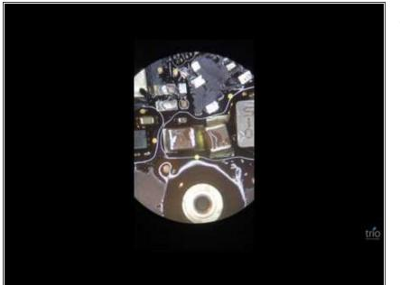
Inspect the Main LogicBord for any sign of liquid exposure. This should be done with a high powered stereo microscope, each SMD component should be checked for any signs of damage. If damage is found logic board should be cleaned ultrasonically and damaged SMD components replaced. This video will show you what MAY be required to repair your MLB.
