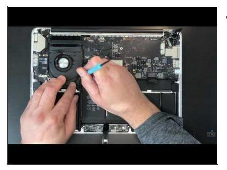
Any MacBook that is exposed to liquid requires a thorough inspection, even a small amount of corrosion untreated can cause a system failure further down the road. You will need to completely disassemble your MacBook to ensure a thorough diagnostic. Here is an idea of what you can expect in a disassembly.
