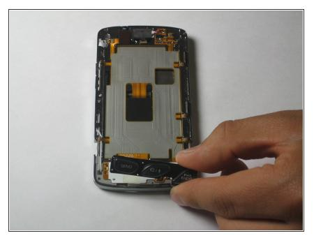
With the phone still facing upwards, identify and remove the three buttons at the bottom end that say "Send", "Clear", and "End." They should come off easily.
