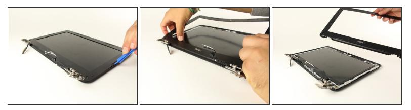
• Using a plastic opening tool to start, and then eventually your hands, pry the front most face of plastic off of the screen assembly.
