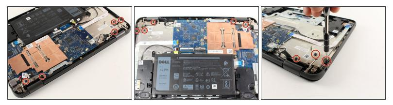
• Using a Phillips #0 screwdriver, remove each of the five 5.5mm screws.
