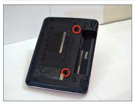
Remove the two countersunk keyboard screws using the Phillips #00 screwdriver.
