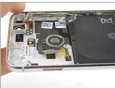
Position your thumb over the fingerprint sensor and push firmly until the sensor pops out of its indention.
