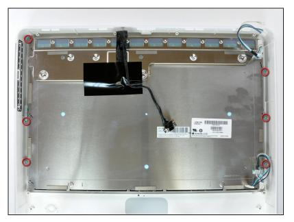
Remove the six 7.2 mm coarsethread T10 Torx screws securing the display to the front case.
