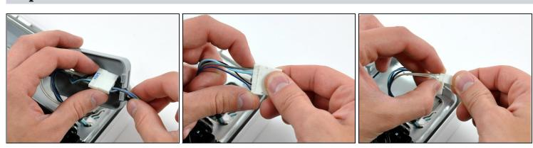
• Remove the inverter cables from the inverter cable cover, and disconnect both connectors.
