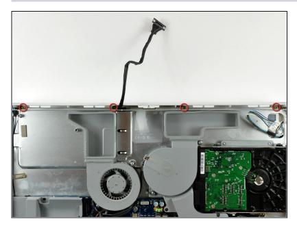
Remove the four coarse-thread
