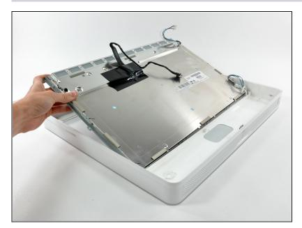
• Lift the display out of the front case.
