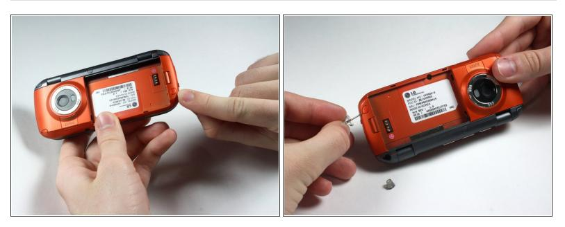
• Remove the 5 screw covers on the back of the phone using a Push Pin.
