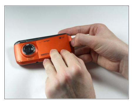
Push/pull the latch away from the camera, causing the battery to pop out.
