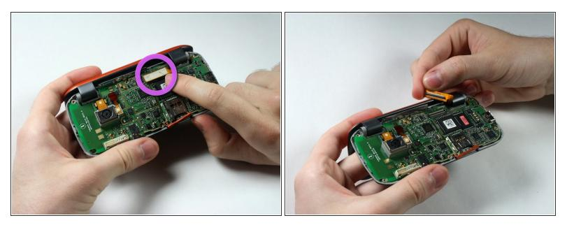
• Gently pry and detach the connection located near the hinge with fingers.
