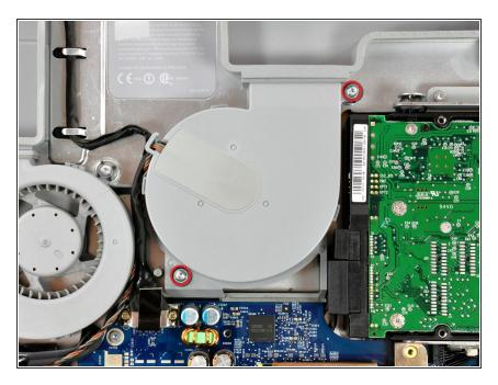
Remove the two 11.6 mm shouldered T8 Torx screws from the right fan.
