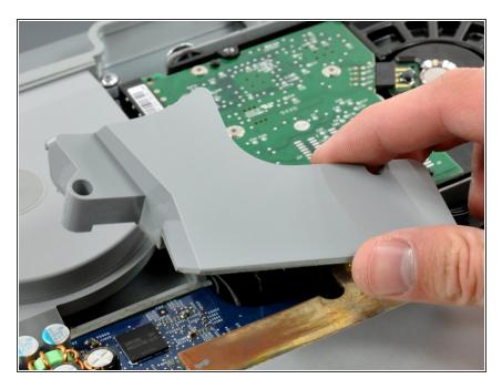
Lift the fan duct out of the chassis.
