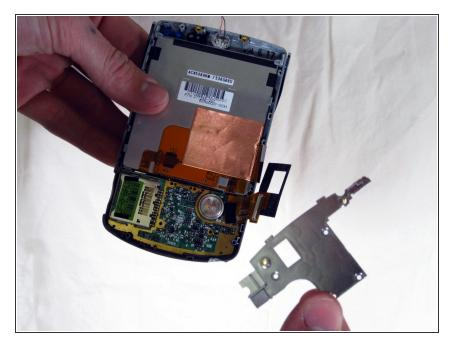
Holding the phone in the same orientation as the photo, gently pull off the backing of the keyboard and place it aside. Removing this backing grants you access to the keyboard.
