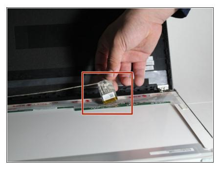
Disconnect the LCD panel from the computer by peeling the connector off.
