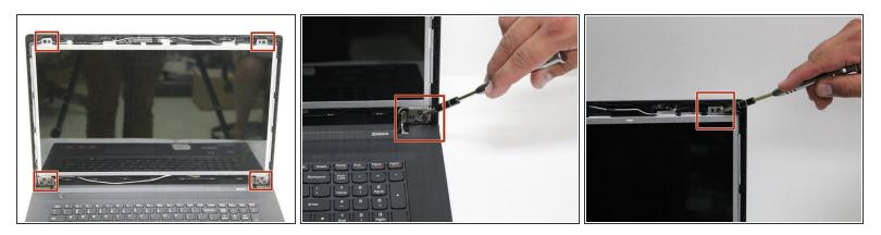
• Use a screwdriver to remove the screws that secure the LCD panel to the computer.
