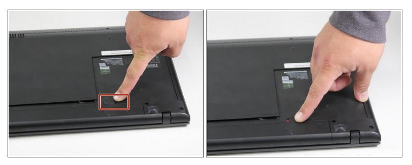
(i) Located directly below the bottom plate will be two switches near where the battery is located.
