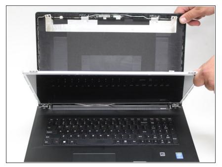
• Carefully separate the LCD panel from the plastic cover, placing it face down on the keyboard
