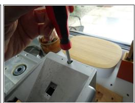
The lid is equipped with four screws, two at the bottom front, two at the back up. One is a Torx 10, the other cross-slot.
