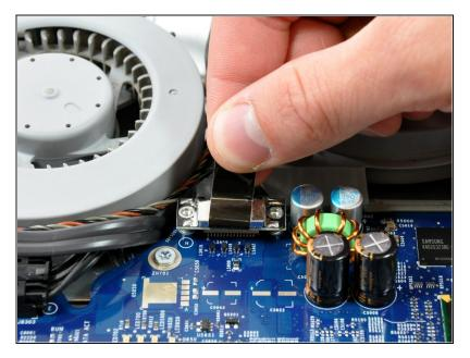
• Pull the display cable up off the logic board by its black pull tab.
