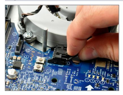
Disconnect the SATA power cable by depressing the lock mechanism and pulling the connector straight away from its socket (parallel to the face of the logic board).
