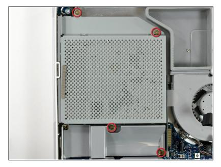
• Remove the four 7 mm Phillips screws securing the optical drive to the midplane.
