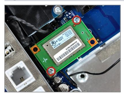
Remove the two 5.5 mm T6 Torx screws securing the Bluetooth board to the logic board.
