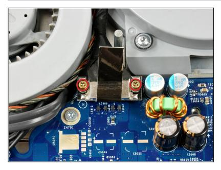
Remove the two 7.3 mm Phillips screws securing the display data cable to the logic board.
