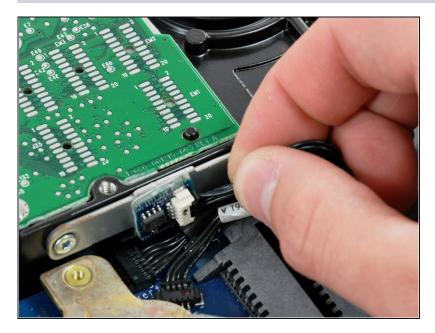
Disconnect the hard drive thermal sensor cable from the hard drive thermal sensor board.
