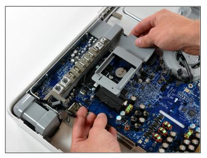
• Gently lift the logic board from its left side to clear the two pins mounted to the midplane.
