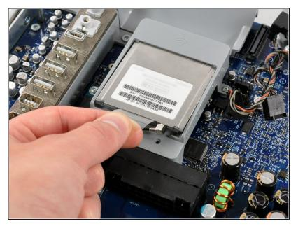
• Lift the AirPort card slightly by its plastic tab and pull it straight away from its socket.
