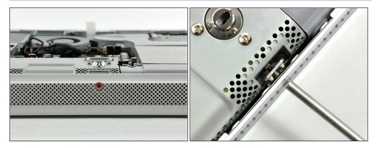
• Rotate the center Phillips screw on the bottom of the iMac clockwise until the rear panel clamp contacts the edge of the case.
