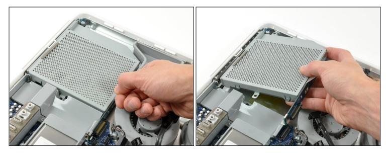
• Pull the optical drive up by its white pull tab to disconnect it from the logic board.
