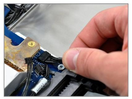
• Disconnect the black inverter cable from its socket on the logic board by pulling the cable straight away from its socket toward the side of the iMac.
