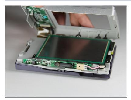
Pry the two halves of the case apart with the opening tool.
