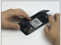
Now that all the screws have been removed, use a plastic opening tool to carefully pry at each of the corners until loosened.
