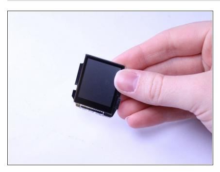
Once free from the Front Casing and the motherboard, you are ready to replace the screen.
