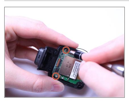
Remove the two 2.0 mm Torx Head screws with the T5 Torx screwdriver.
