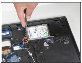
• Using your Phillips Screwdriver, remove the four screws around the hard drive.
