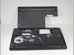
Remove the two placeholder screws, and then proceed to pull off the back of the laptop.
