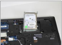
Shift the hard drive to the right and you will feel it click. That means it has been unlocked and can be removed.
