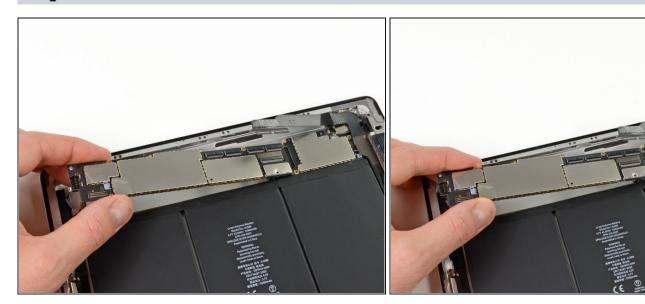
Holding the logic board by the side nearest the dock connector, carefully pull the logic board toward the bottom of the iPad.
