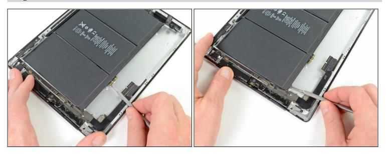
• Continue releasing the adhesive near the top of the battery.
