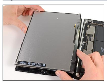
Without touching the front of the LCD, lift the LCD off the front panel.
