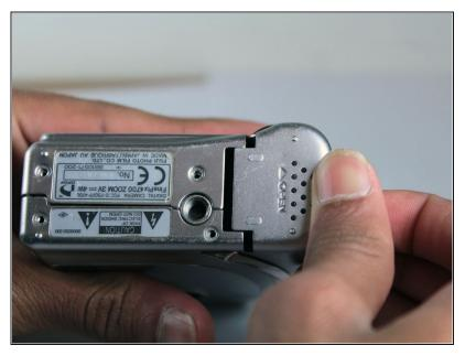
Slide open the battery compartment cover with your thumb.
