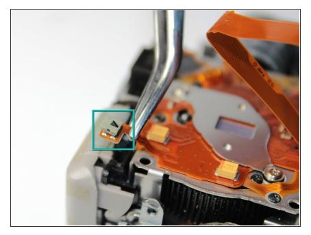
Use the tweezers to pull gently on the small orange ribbon, located in upper left hand corner near the flash, to remove the square insert.
