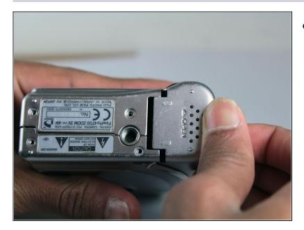
• Slide open the battery compartment cover with your thumb.
