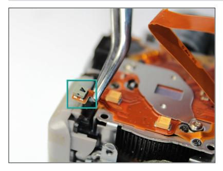
Use the tweezers to pull gently on the small orange ribbon, located in upper left hand corner near the flash, to remove the square insert.
