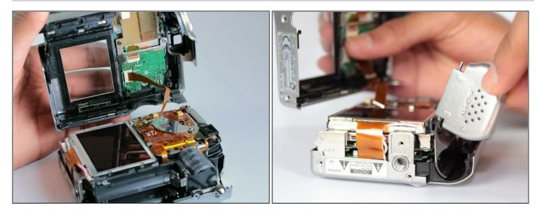
A Watch out for the orange ribbon that is still attached to the back cover when you lift it up. It is very delicate and might rip.
