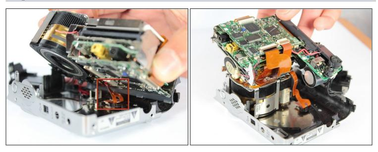
⚠ Do not fully separate the motherboard unit from the front cover. There is still a ribbon attached and it will rip.
