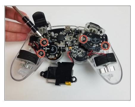
Unscrew the four 9mm Phillips #0 screws that are attached to both joy stick control mini-motherboards.
