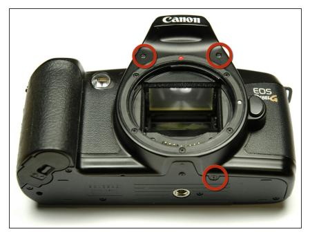
Using a #00 Phillips screw driver, remove three 4.4 mm Phillips screws as indicated by the red circles.
