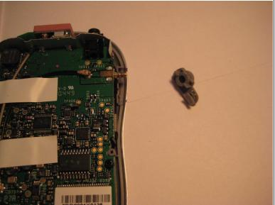
Remove the plastic antenna extension connector on the right side of the device.
