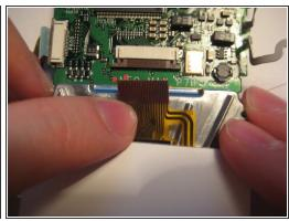
To remove the ribbon cable from the board, catch the sides of the connector with fingernails and pull downward.
