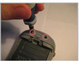
Remove the two screws under the button using the T6 Torx screwdriver.
