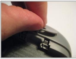
Remove the button cover on the back of the device by prying it up with a spudger or your thumb nail.
