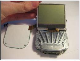
Pivot the LCD screen, pulling on the top and sides and keeping the bottom attached.
