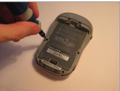
Remove the four screws from the bottom of the device using a T6 Torx screwdriver.
