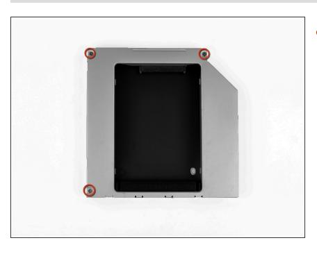
Remove the three 3.0 mm Phillips screws from the optical bay enclosure.
