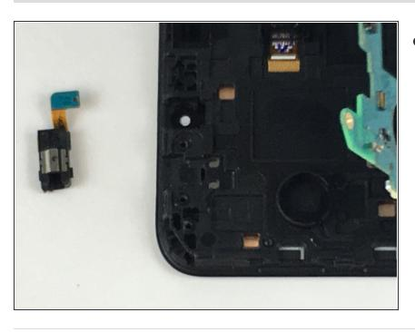
Remove the auxiliary port from the case.
