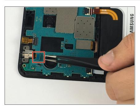
Using tweezers disconnect the headphone jack connector from the motherboard.
