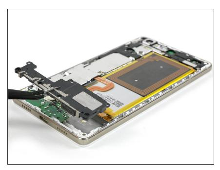
Remove the loudspeaker carefully.
