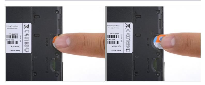
Slide out and remove the SIM card.
