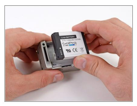
Remove the battery from the case.
