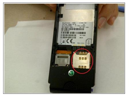
Slide the SIM card into the lower right slot identified by the circle in the picture, ensuring the contacts are aligned properly.
