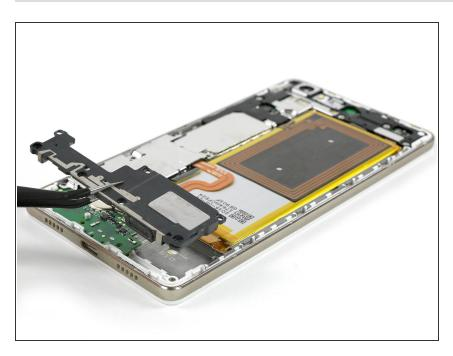
Remove the loudspeaker carefully.
