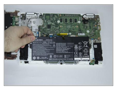
Remove the battery by pulling upwards.
