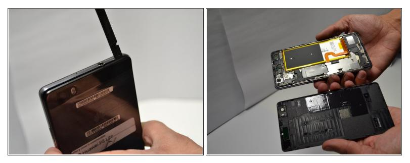
• Begin by removing the back cover of the device with the <u>Spudger</u>. To prevent damage to the back cover, begin removing the cover half an inch to the right of the headphone jack and continue prying around the perimeter of the device.
