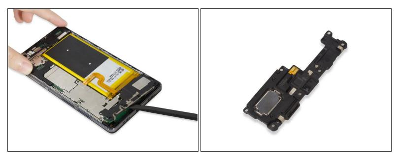
Use the <u>Spudger</u> to gently remove the Loudspeaker from the device. Place the replacement Loudspeaker into the device.
